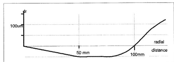
MK4 radial symmetric lens distortion determined by selfcalibration Hildesheim
