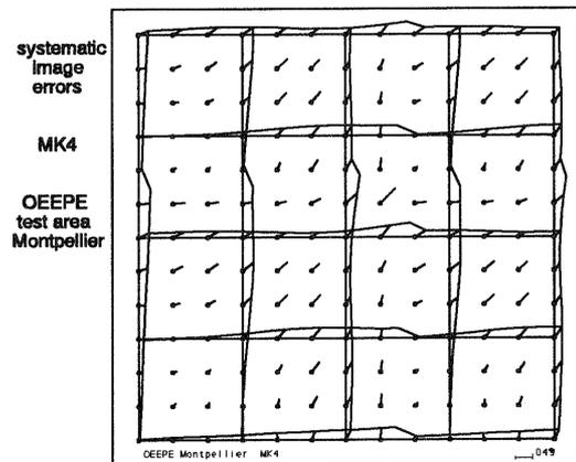
**Figure 4:** systematic image errors of the MK4
