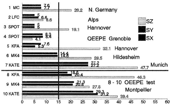
**Figure 3:** accuracies of independent check points determined by bundle adjustment [m]
