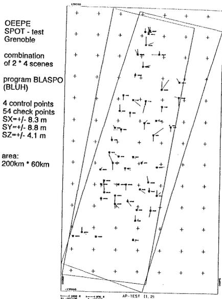
**Figure 6:** results of the block adjustment of a combination of 2\*4 SPOT scenes
