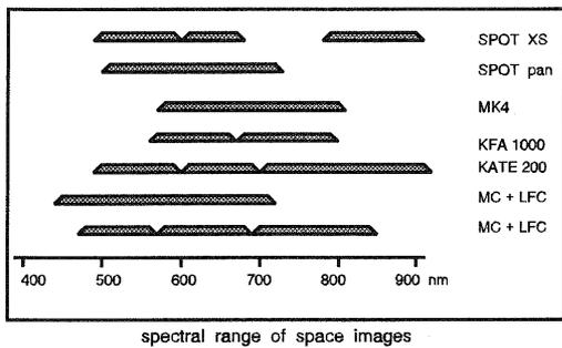
**Figure 2:** spectral range and resolution
