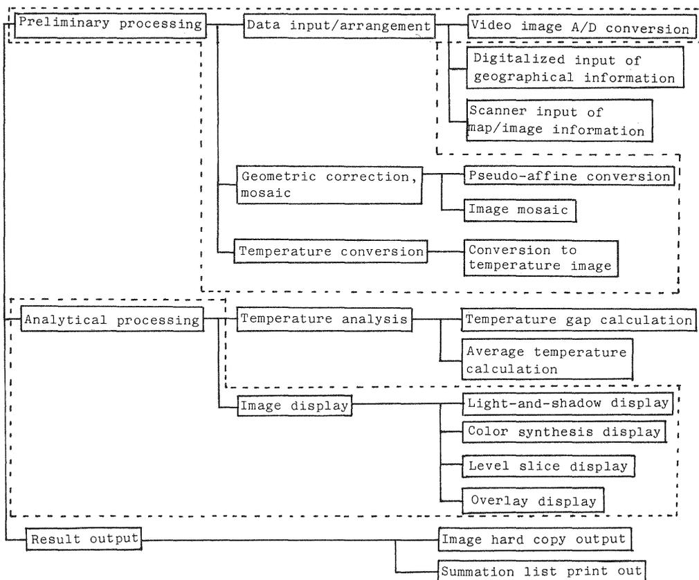
Fig. 6 Software configuration
