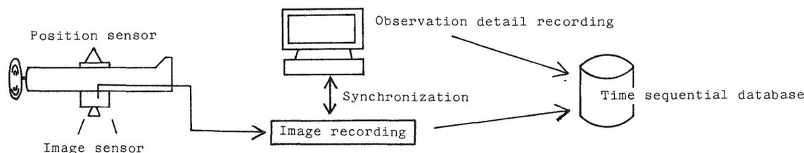
Fig. 3 Concept of time sequential database at the time of observation
