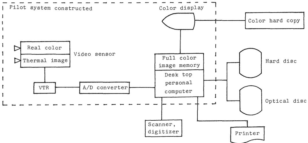
Fig. 5 Hardware configuration
