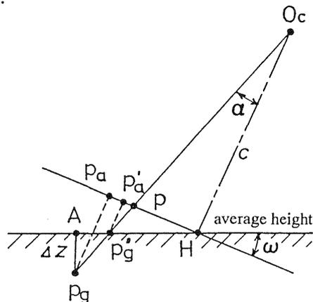
Figure-5 : image transformation error due to height difference in the terrain
