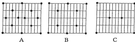
Figure-9b : configurations of control and check points in the analysis of satellite CCD line-scanner imageries taken oblique to the flight paths
