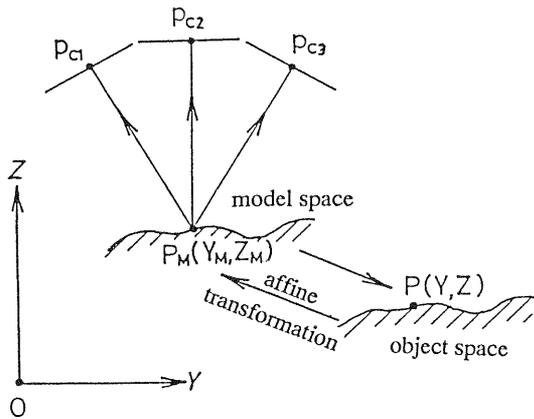
Figure-2 : relative and absolute orientation of three overlapped affine line images
