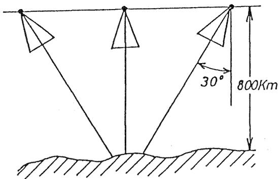
Figure-6 : three overlapped CCD line-scanner imageries taken from the three different flight paths of the satellite
