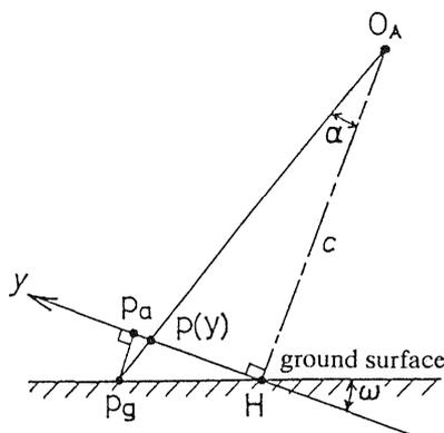
Figure-4 : transformation of a central-perspective line image into an affine one
