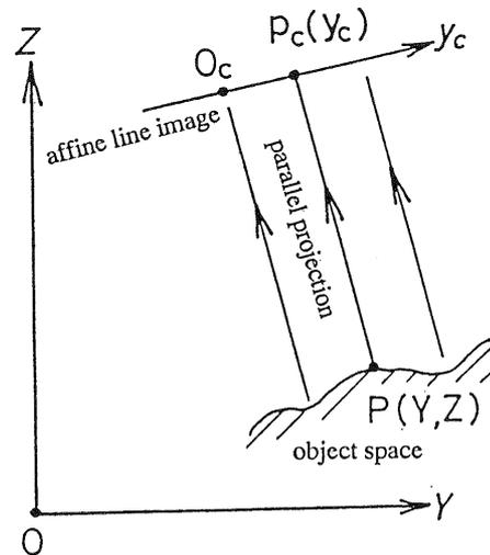
Figure-1 : parallel projection of an object space into a line in a plane
