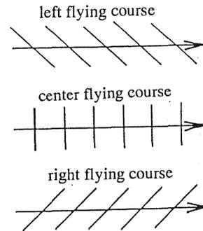
Figure-7 : three overlapped CCD line-scanner imageries taken oblique to the flight paths
