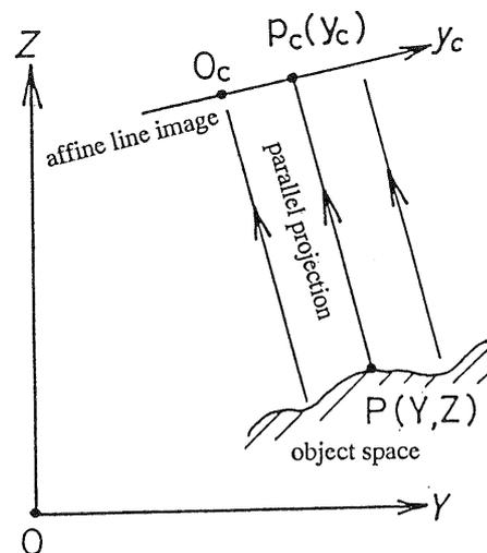
Figure-1 : parallel projection of an object space into a line in a plane
