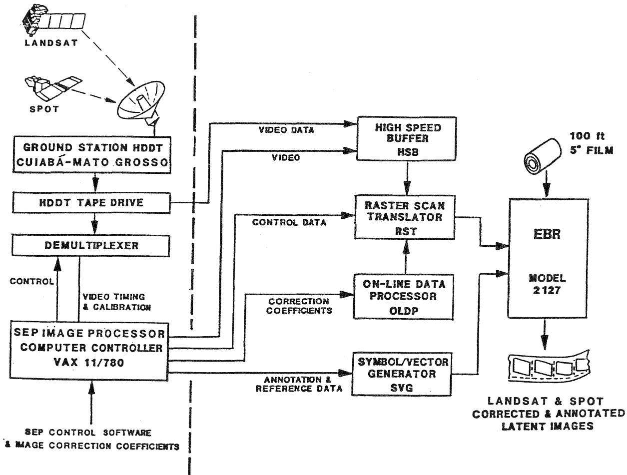
FIGURE 2 EBIR System for Image Processing Subsystem LPI Cachoeira Pulista INPE, Brazil
