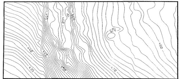
**Fig. 8.5 - Representation with contours line of the surface smoothed manually**
