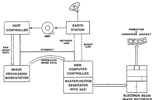
Figure 1 EBIPS-3000 System Configuration
