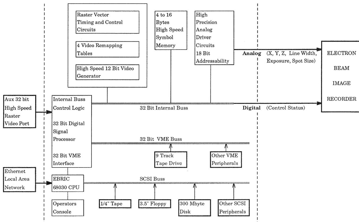
Figure 2 Block Diagram of RVG 450
