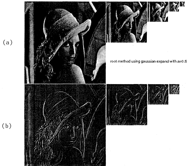
Figure 3. The first five levels of (a) the Gaussian pyramid and (b) the Laplacian pyramid of the image 'Lena'.
