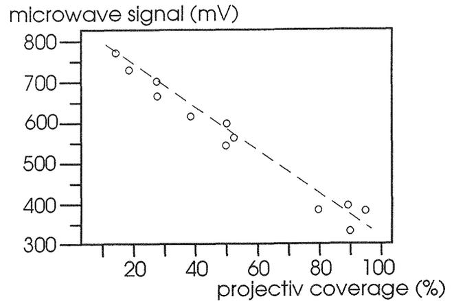
fig. 3: Microwave radiometer signal as function of the ground coverage on flooded rice fields.
