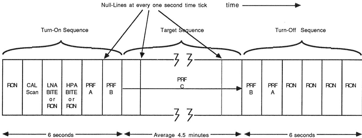
Figure 1: SIR-C input data run format. Each segment in turn-on and turn-off sequence is 1 second duration.
