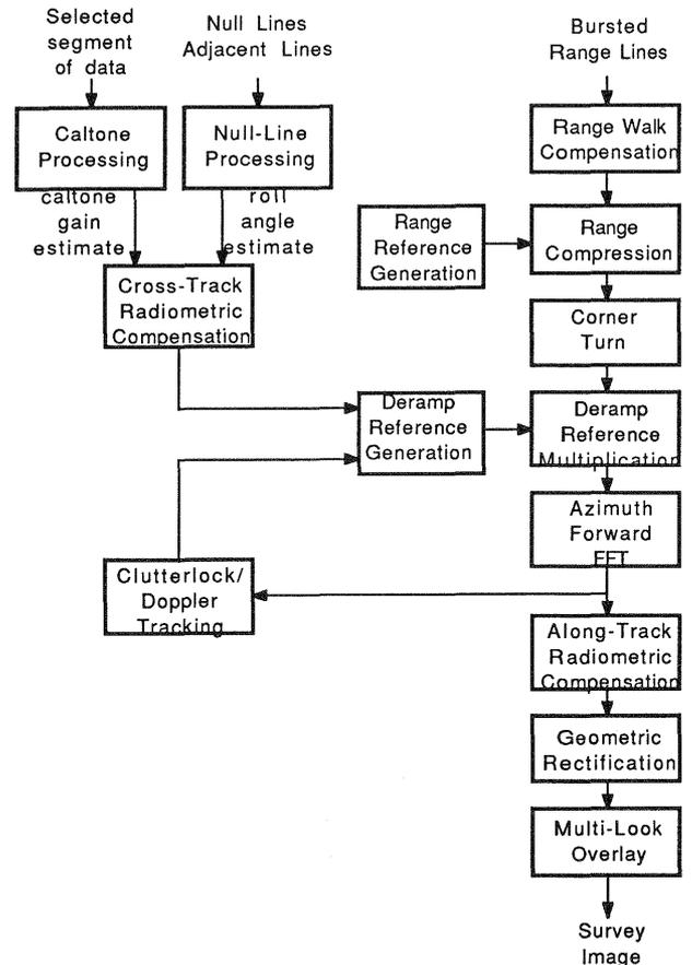
Figure 2: Survey processing algorithm flowchart.
