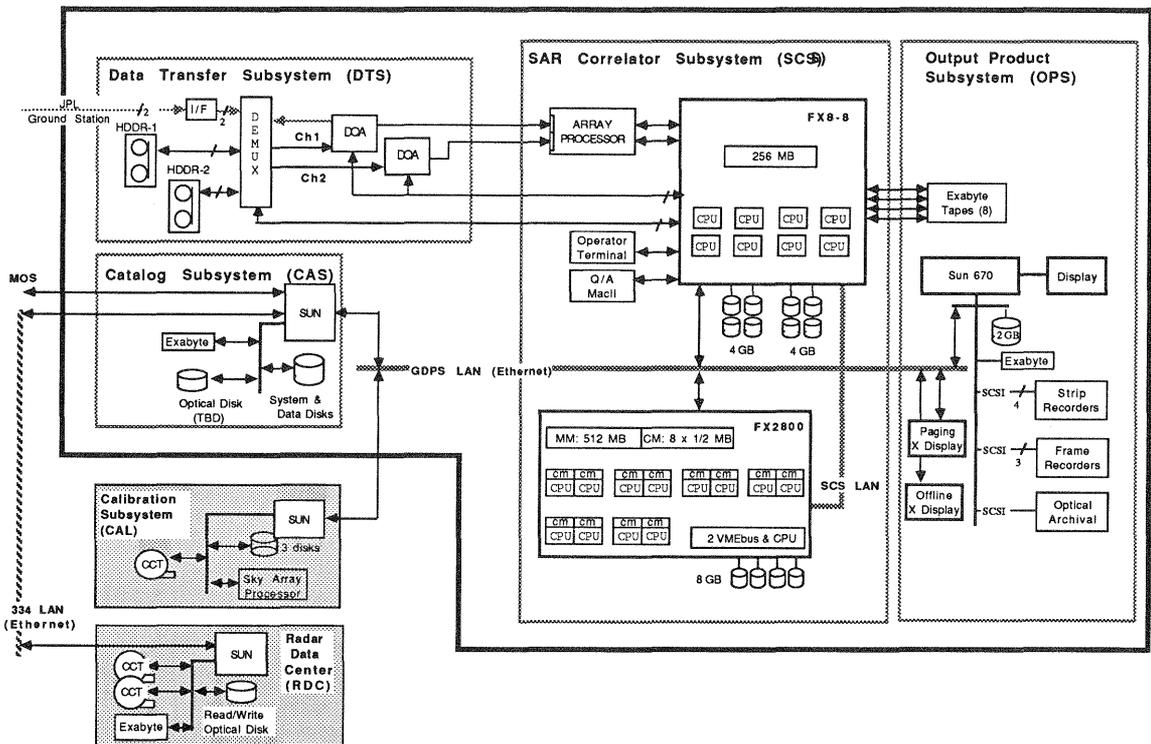
Figure 4: SIR-C ground data processing system hardware architecture.
