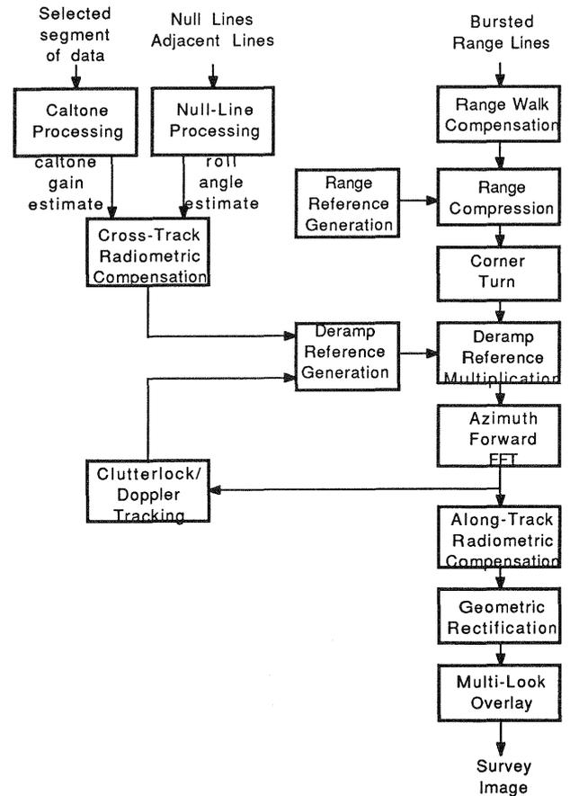
Figure 2: Survey processing algorithm flowchart.
