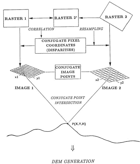
Figure 1: Scheme of automated stereo mapping
