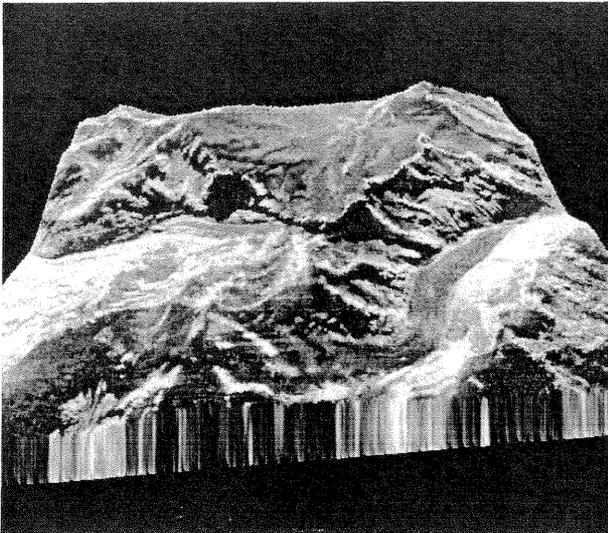
Figure 11: Superposition of stereo-derived DEM and SAR image data.
