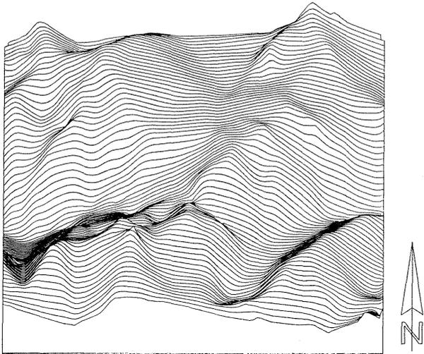
Figure 5: Axonometric oblique view of the stereo-derived DEM.
