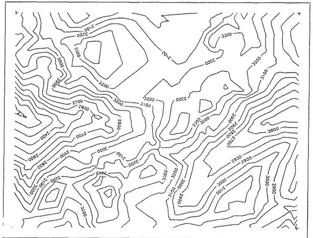
Figure 8: Contour line plot of the stereo-derived DEM (contour interval 100 m).
