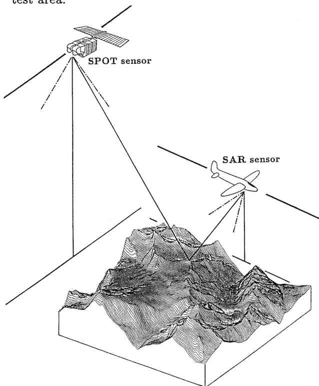
Figure 2: Stereo configuration given by SAR and SPOT image acquisition geometry.
