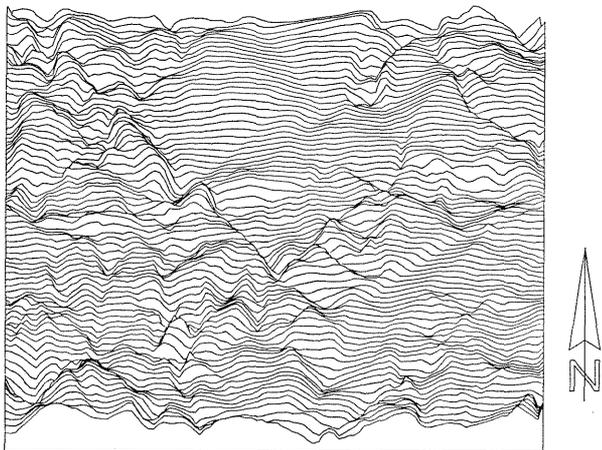
Figure 7: Axonometric oblique view of the difference DEM.
