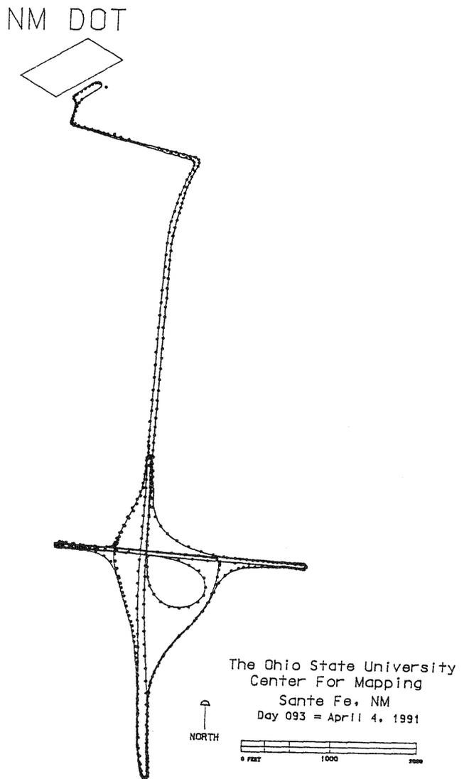
Figure 2: Resulting alignment of a combination of inertial and GPS observations. The circles indicate position fixes by GPS.
