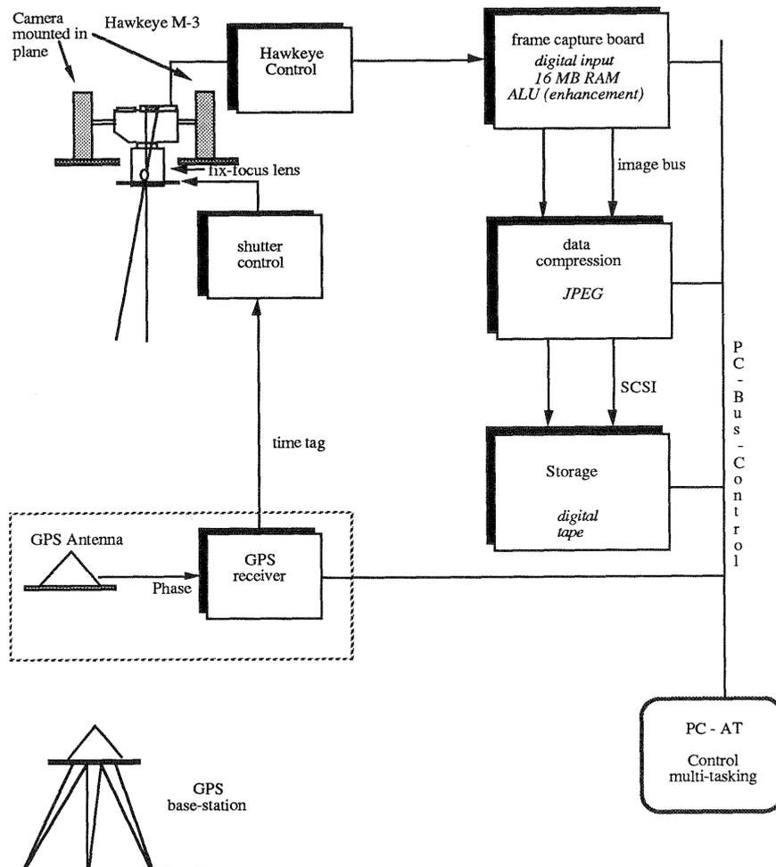
Figure 6: The system chart of the GPS controlled digital high-resolution mapping system (MAPCAM).
