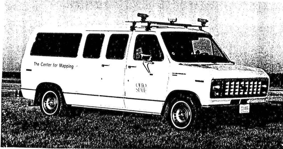
Figure 3: The GPS-Van which combines GPS, inertial navigation and stereo-vision technologies with GIS.
