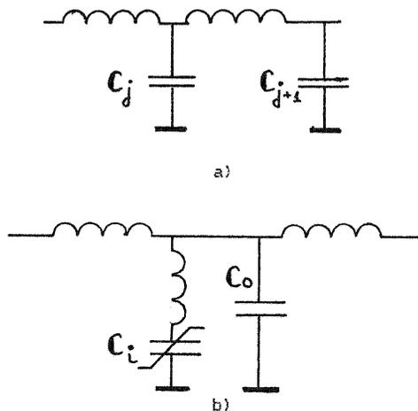
Figure 4. Electrical model of neuronlike network
