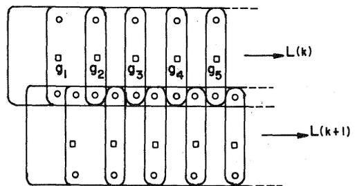
Figure 13. Shift of strips: arrangement of photographs, tie points and models,  $p=60\%$ ,  $q=20\%$ .
