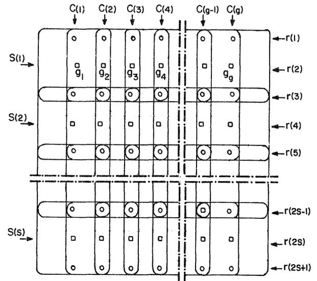
Figure 3-1. Set up of photographs and tie points,  $p=60\%$ ,  $q=20\%$ .
