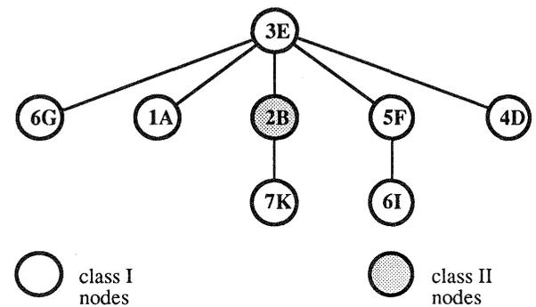
Fig. 5.2. The propagation tree. Even though the edge segments 2 and B do not seem to match very well (see difference in direction), match (7, K) was found.
