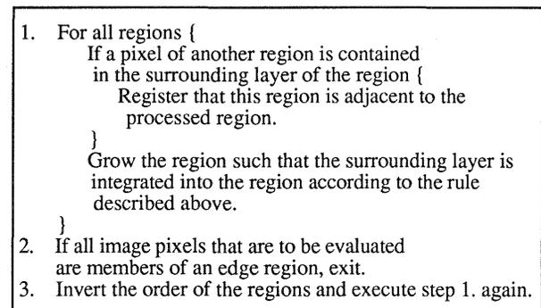
Fig 4.1. Algorithm for the generation of a Region Adjacency Graph.
