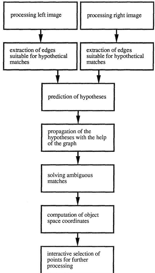
Fig. 1.2. The matching procedure. Graph-based matching and derivation of object space coordinates.
