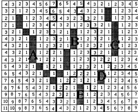
Fig. 4.2. Final state of the region growing by layers. The edge segment pixels are shown in gray. The labels surrounding the edge segments are the layer indices. The bold lines are borderlines between edge regions. Next neighbours are A-B, A-E, B-C, B-D, B-E, C-D and D-E.
