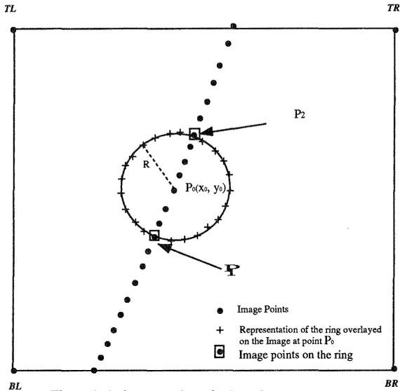
Figure 1. A ring around a point P and a line crossing the ring at two points
