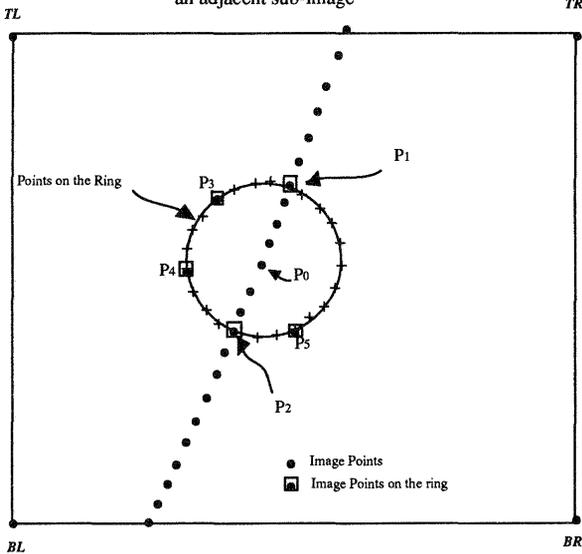
Figure 3. A ring around an image point P. Points that are on the ring are stored in array Bound
