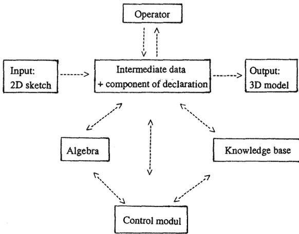
Fig. 6 Components of the rule-based system
