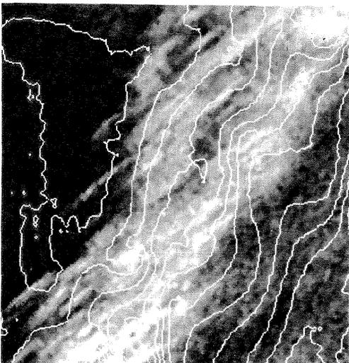
Figure 5. Contour lines derived from the reconstructed seafloor surface by shape from shading technique
