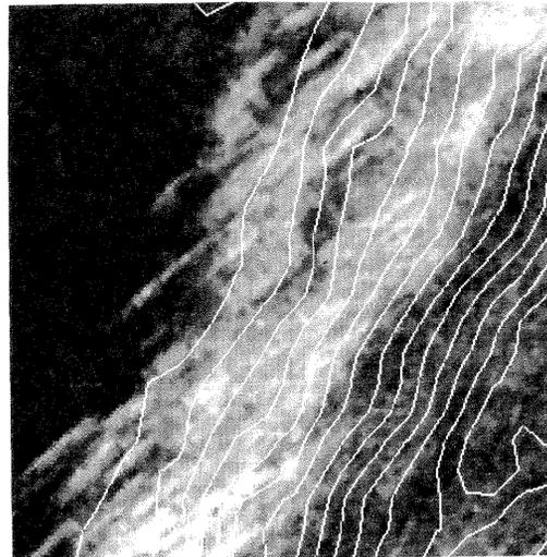
Figure 4. Contour lines derived from SEA BEAM bathymetric data in the same area covered by the sonar image in figure 3
