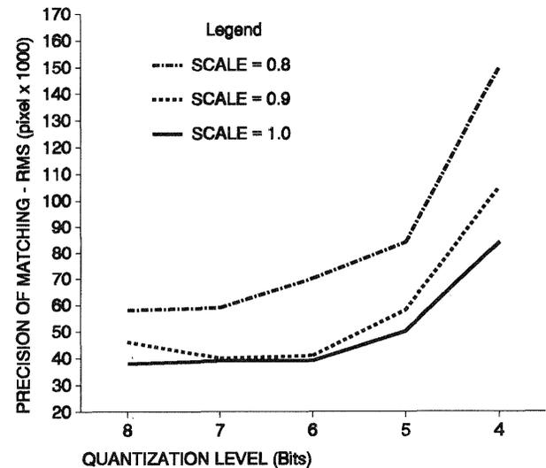
Figure 3 Precision of least squares matching in terms of quantization level for circular feature 100  $\mu\text{m}$  in size, for 3 cases of scale variations between the two images, and pixel size of 12.5  $\mu\text{m}$ .
