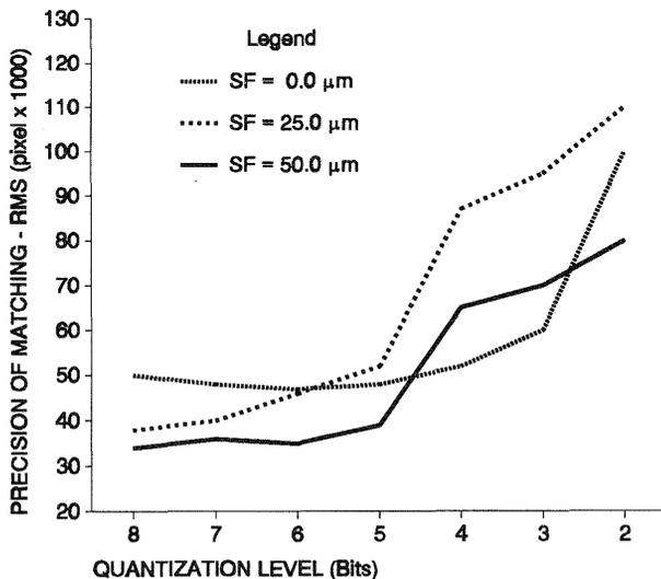
Figure 1 Precision of least squares matching for circular feature 100  $\mu\text{m}$  in diameter, in terms of quantization level for 3 spread function sizes (SF) for pixel size of 12.5  $\mu\text{m}$ .
