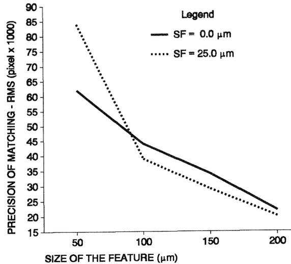
Figure 2 Precision of least squares matching in terms of circular feature size for 2 spread functions (SF) and pixel size of 12.5  $\mu\text{m}$ .
