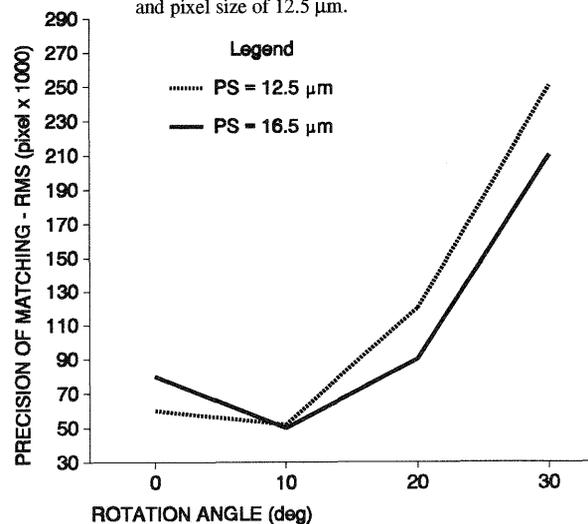
Figure 4 Precision of least squares matching in terms of crosses with 3 cases of rotations between the two images, and pixel size of 12.5  $\mu\text{m}$ .
