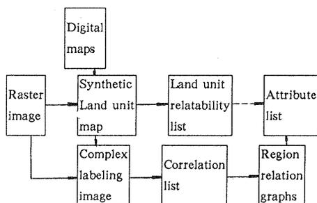
Figure 2. Multilevel representation tree
