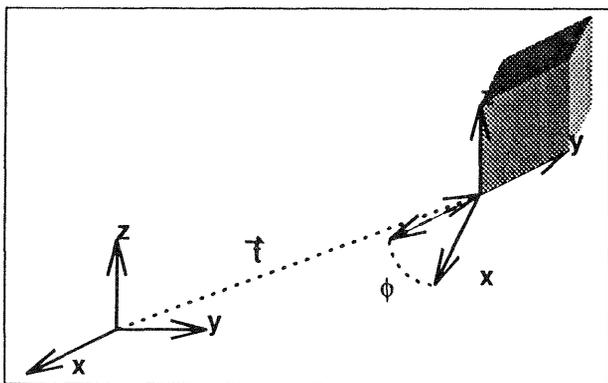
Figure 3: Position and orientation parameters for a body:
