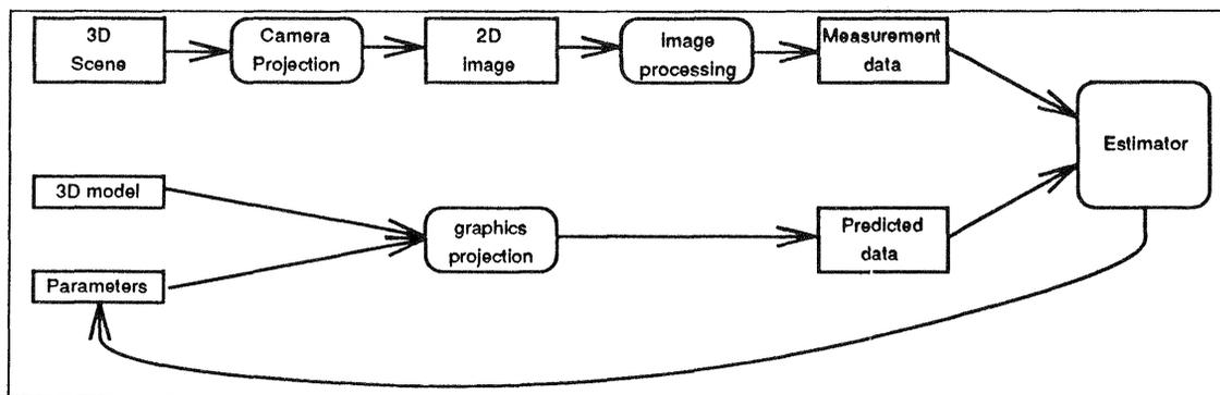
Figure 2: Diagram describing the iteration loop of the parameter estimation, applied to image data.
