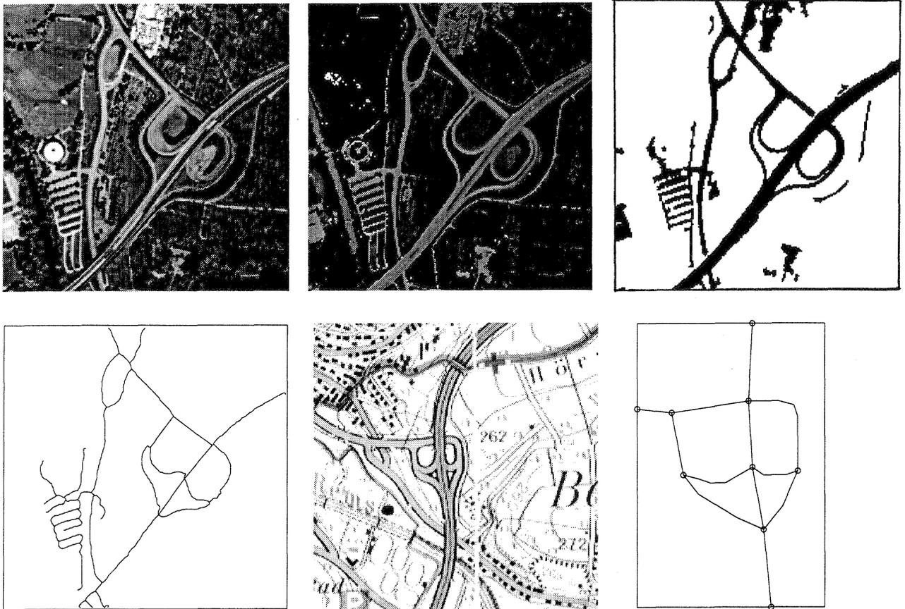
Figure 1: Example street1: intensity image (top left), hue image (top middle), binary image (top right), extracted image lines (bottom left), map (bottom middle), landmark model (bottom right)
