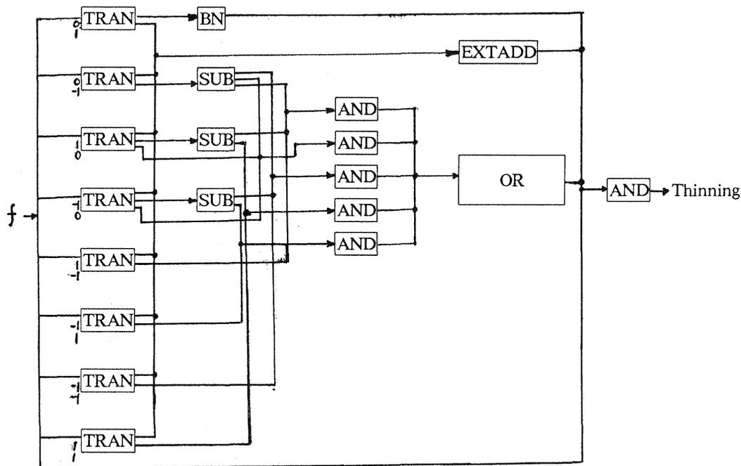
Fig. 1 Block Diagram for Image Thinning
