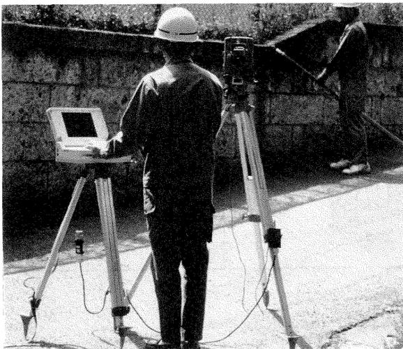
Photo 2.4 Field Supplementary Surveying using CG Plane Table Surveying system
