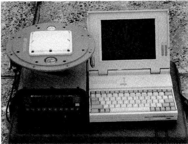
Photo 2.8 Real time GPS mapping system
