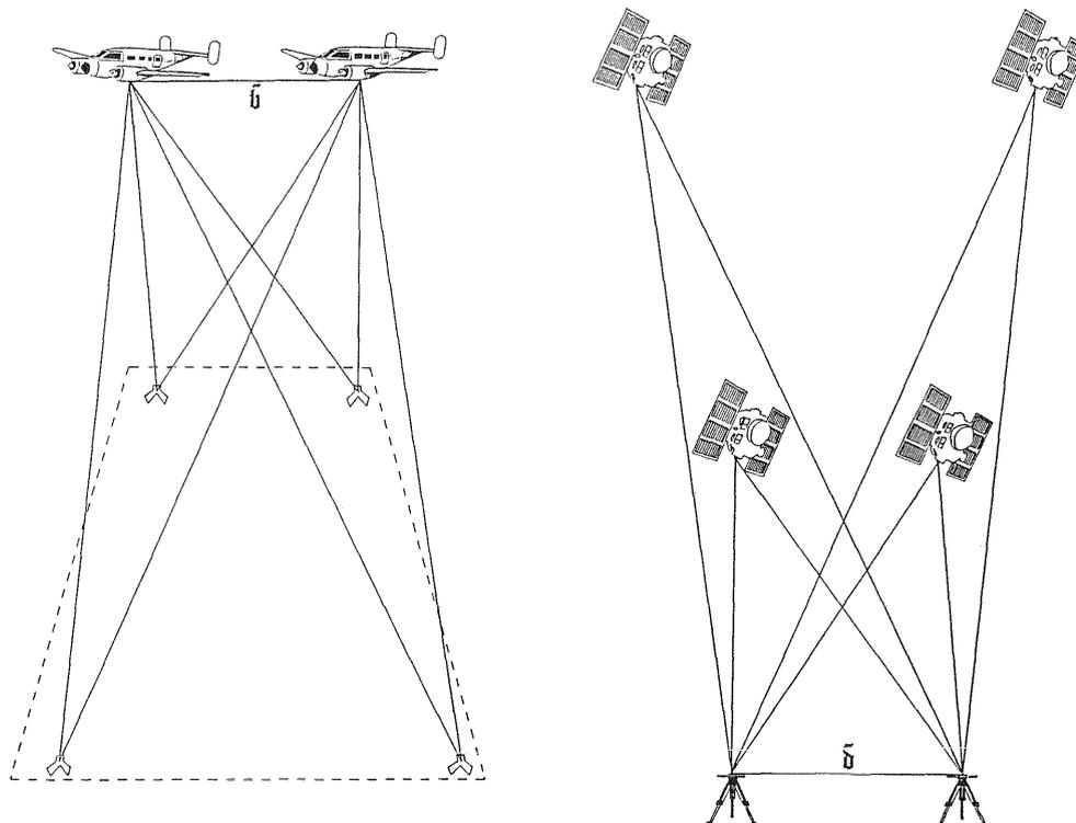
Figure 1. Photogrammetry and GPS - kinship in figuration
