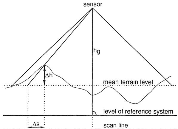
Fig. 2: Displacements  $\Delta s$  caused by terrain height differences  $\Delta h$
