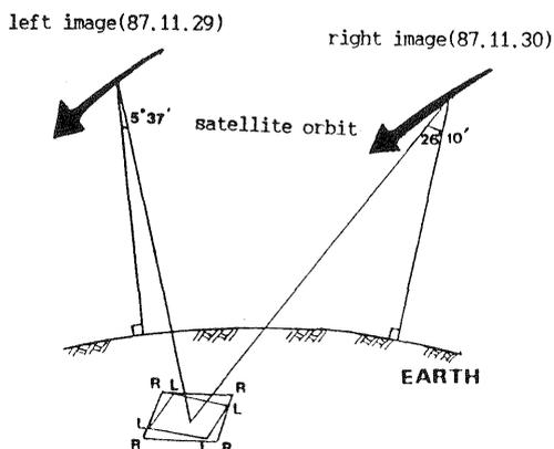
Fig. 3 stereo model of satellite images
