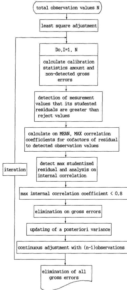
Fig. 2 flow of progressive data snooping method
