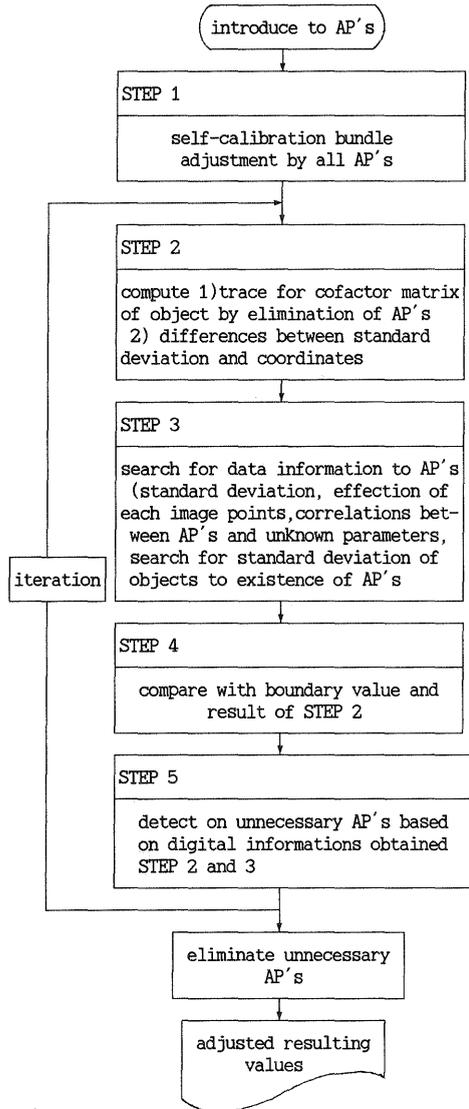
Fig. 1 determinability test of AP's
