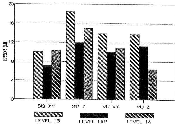
Fig. 5 3-D positioning accuracy with preprocessing
