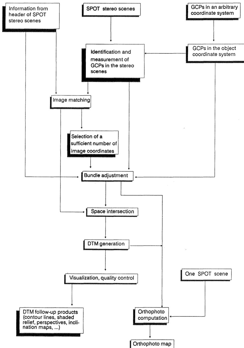
Fig. 1: Photogrammetric processing of SPOT images, data flow
