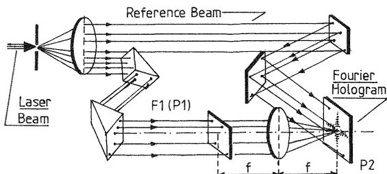
Fig.2. Optical assemblage for obtaining Fourier hologram
