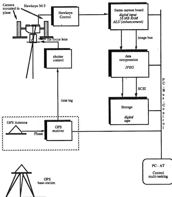
Figure 2: Layout of the complete MapCam system.
