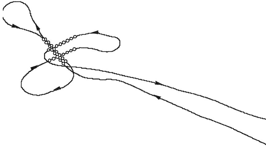
Figure 4: Flight-lines of the first test-flight after differential GPS processing. The images are marked by circles.
