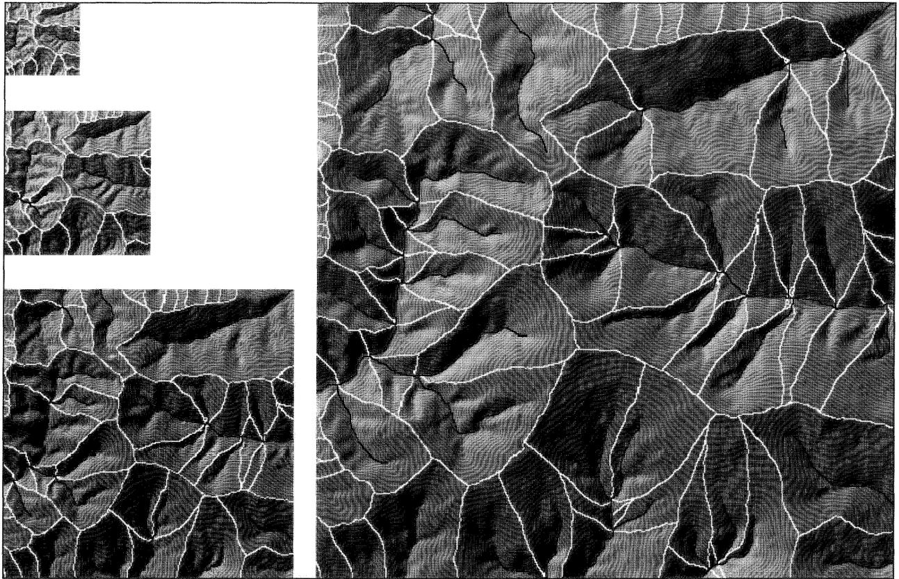
Fig. 11: Test region in 4 levels: 61x61 grid-cells with 200m grid width; 121x121 cells (100m); 241x241 (50m); 481x481 (25m).
