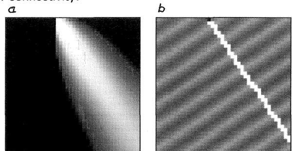
Fig. 2: Drainage in a slope. a) Drainage quota values (DQV) highlighted; b) Path of maximum DQV's on contour-bands (dark gray lines against light gray zones).
