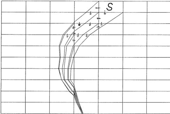
Fig. 3: Splitting of drainage channels in the grid. **S** is the starting cell, the arrows show transitions of water. The channels arise from the edge points around the grid-cells.
