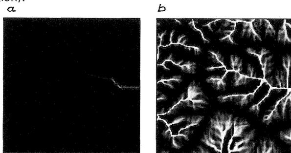
Fig. 6: Drainage accumulated by the ordered calculation in a part of the model of fig. 4. a) Values as calculated: White means much water (maximum: appr. 5850 units), black little water. b) Values after a histogram equalization.
