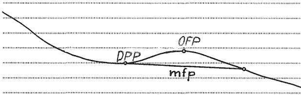
Fig. 1: Pit and main flow path (mfp), longitudinal section. DPP: Deepest pit point; OFP: Outflow point
