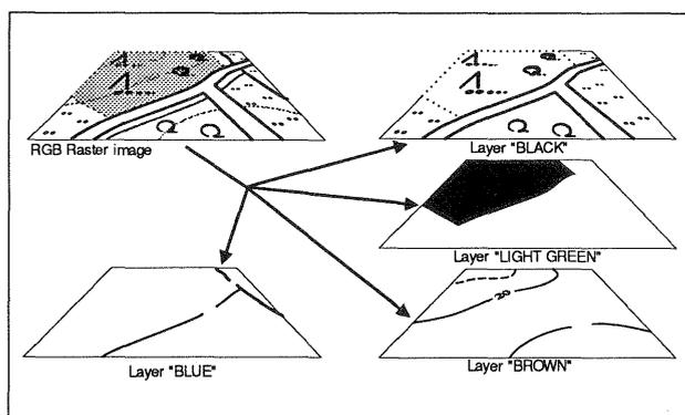
Fig. 3: Separation of color layers.
