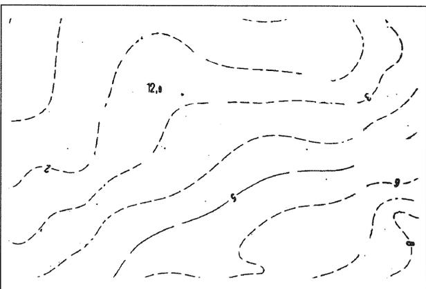
Fig. 12: Color layer BROWN separated from image shown in Fig. 11.
