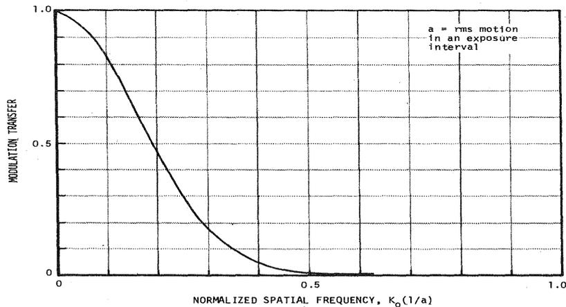
Fig. 1 Attitude jitter is random (Normal distribution) image motion within an exposure time, MTF of the imaging system is degraded
