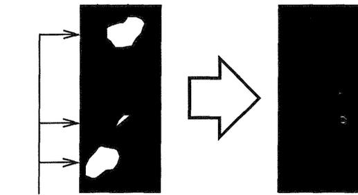
Small isolated holes in a thresholded area
