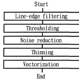
Fig. 4. The flow chart of line edge detection in hierarchical edge detecting algorithm
