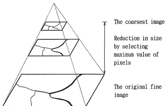
Fig. 3. A series of images structured hierarchically
