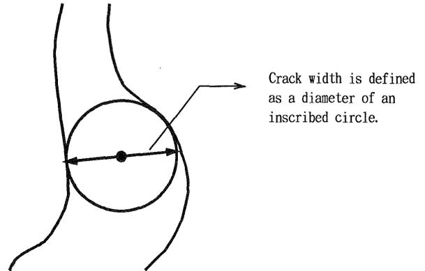
Fig. 11. A definition of crack width
