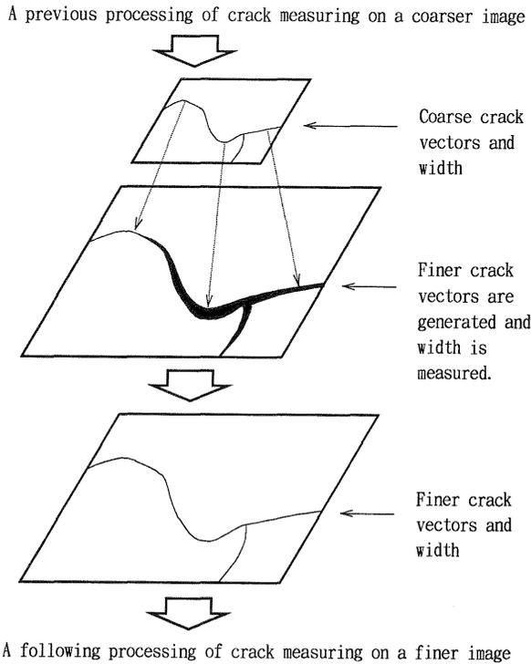
Fig. 5. A schema of hierarchical crack measuring
