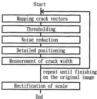
Fig. 6. The flow chart of hierarchical crack measuring algorithm
