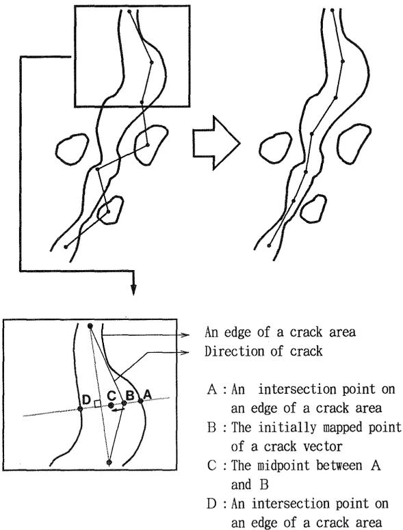
Fig. 10. A schema of detailed positioning by centering
