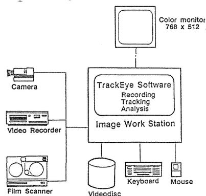
fig 3 TrackEye motion analysis system
