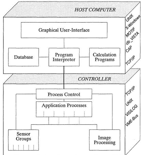
Fig.3 POM software structure
