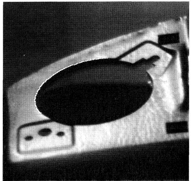
Fig. 6. Measurement of circular loudspeaker hole
