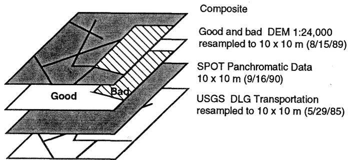
Figure 4. A geometric reliability diagram summarizing data sets and the degree of resampling.
