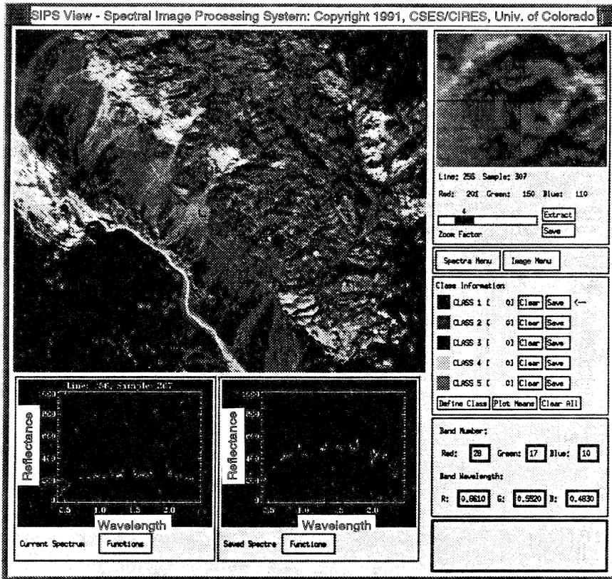
Figure 2. The Spectral Image Processing System (SIPS) graphical user interface is capable of displaying "hyper-spectral" remote sensor data (i.e. more than the standard 1-8 bands). In this example bands 28, 17 and 10 are used in the RGB color planes respectively. A comparative evaluation of the spectral signature of a pixel at an x, y location can be made with a saved spectral signature file. (Courtesy of Dr. Alexander Goetz, University of Colorado, Boulder, CO).
