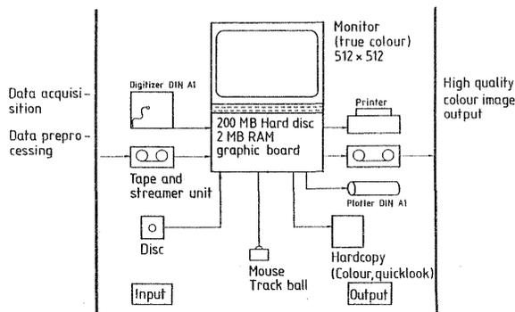
Fig. 5 Hardware configuration for a Data Processing Unit
