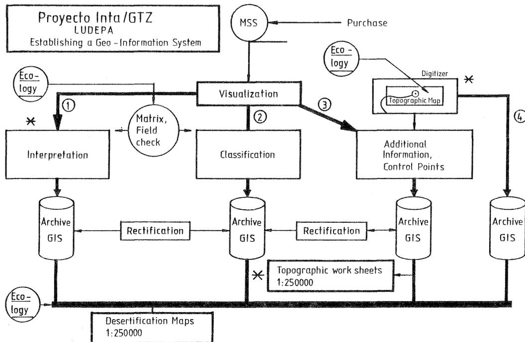
Fig. 4 Data Acquisition in Transects for a GIS Data Base „Desertification Control in Patagonia“
