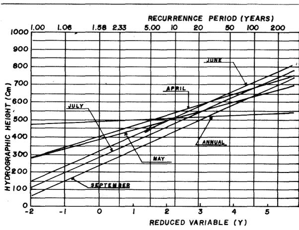
Fig. 2 - Inundation recurrence periods for the rio Miranda at Tição de Fogo.
