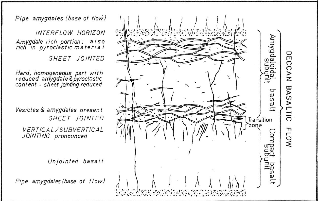
**FIG. 2 :** Schematic vertical section of a typical Deccan Trap basalt flow. The interflow horizons (wherever present) separate successive flows. The subdivisions of the flow described on the left of this sketch are based on petrological considerations. The subunits on the right are based on the hydrogeological characters (modified after Kulkarni, 1987; Kulkarni and Deolankar, 1990). The relative thicknesses of any of the subdivisions vary significantly from flow to flow.
