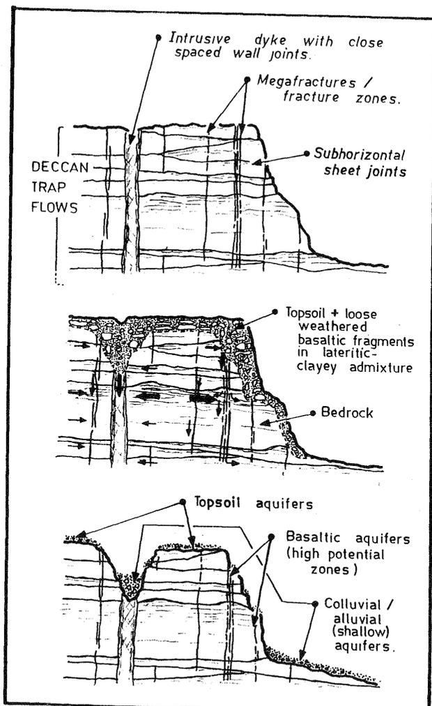
FIG.3 : Schematic sequence of the geomorphic evolution of a Deccan Trap flow pile (modified after Peshwa and Kale, 1988). Note the uneven and irregular nature of individual flows. Arrows in the middle profile represent the movement of water through these flows, and are depicted proportional to the transmissivity of the basaltic rock in the relevant direction.
