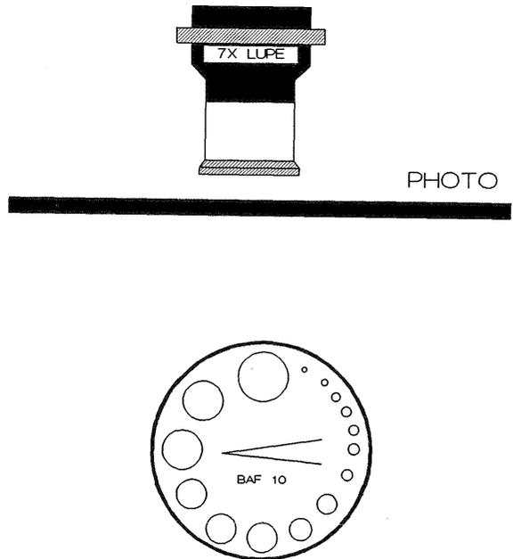
Figure 7. Sample trees are determined using a 7X-power monoscopic comparator with a recticle illustrating the sampling angle (BAF 10). A series of circular diameters is used to estimate tree crown diameter.
