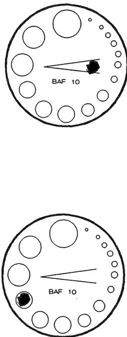
Figure 8. The tree crown that subtends an angle larger than the angle-gauge is counted as an "in" tree and is included in the sample. The crown diameter is estimated using the circle that most closely approximates it and is converted to meters using the photo scale.
