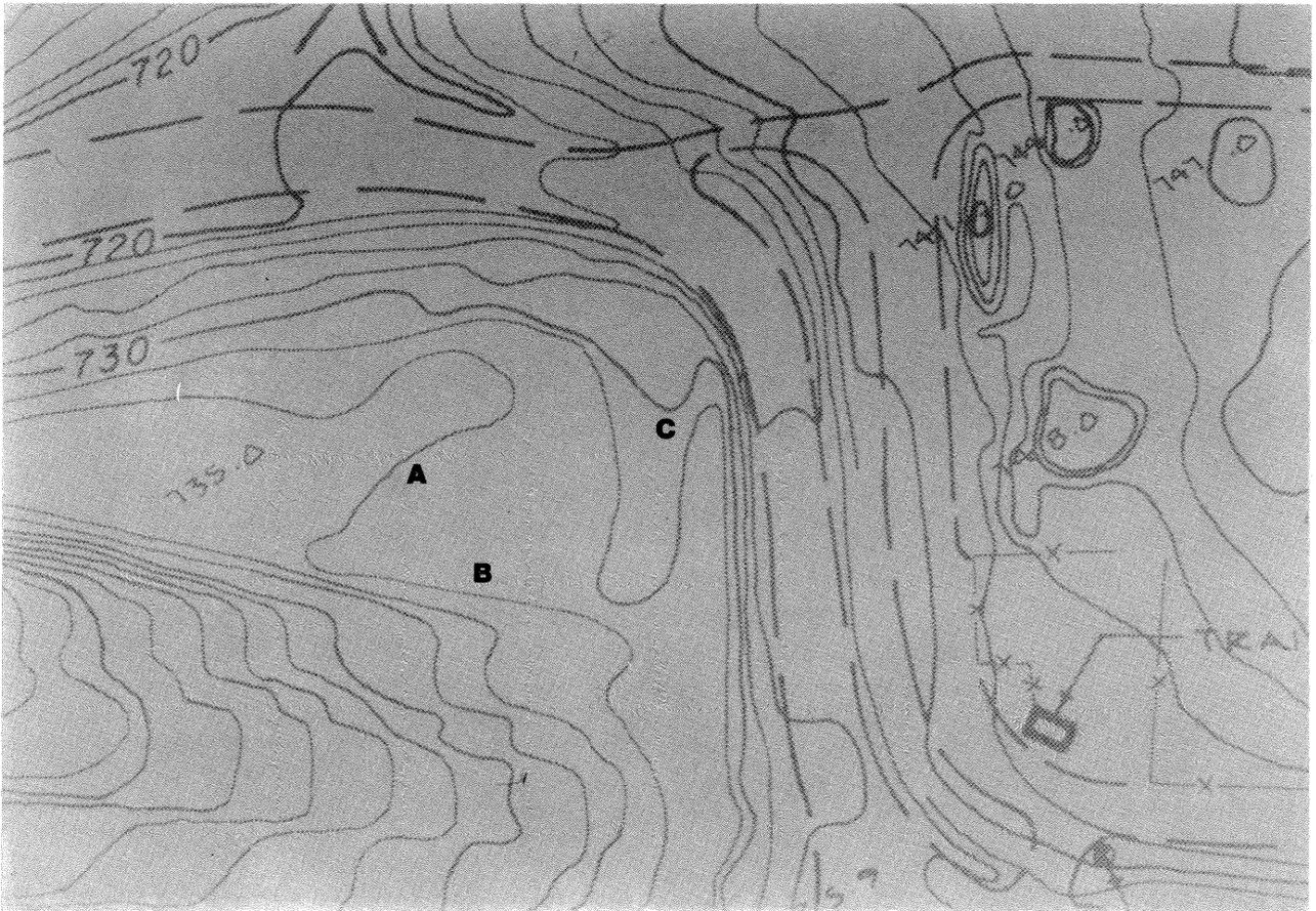
Figure 1. Portion of a 2-foot contour interval topographic map of a landfill in east central Illinois. Three depressions, A, B, and C, found by photointerpretation are shown on the map.
