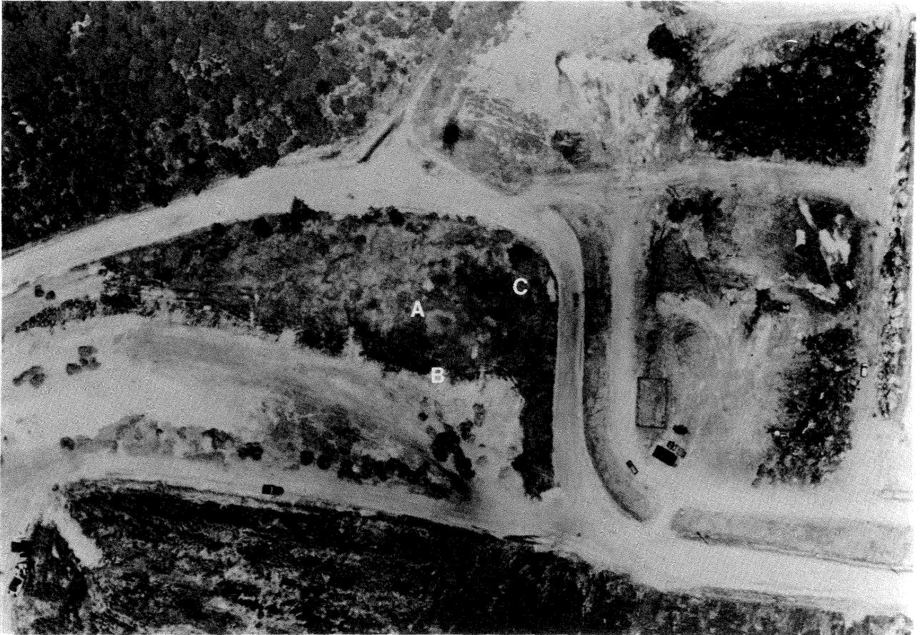
Figure 2. A black and white copy of a color infrared aerial photograph of a closed landfill in east central Illinois, USA. The photo recorded on 18 June 1991, shows 3 depressions, A, B, and C, on the landfill cover found by stereoscopic photointerpretation.
