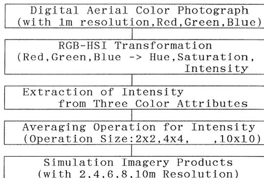
Fig.2 The Procedure for Resolution simulation
