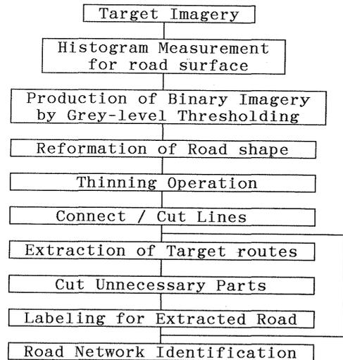
Fig.5 The procedure for Road Network Extraction
