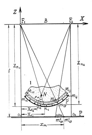
The stereoroentgenography is carried out by means of successive work of the tubes. First the left X-ray tube is switched on, its focus is located at Point  $F_1$ . After the reloading of the flat and flexible film-holders Survey Object 1 is photographed for the second time by means of the right X-ray tube, whose real focus is located at Point  $F_2$ .
