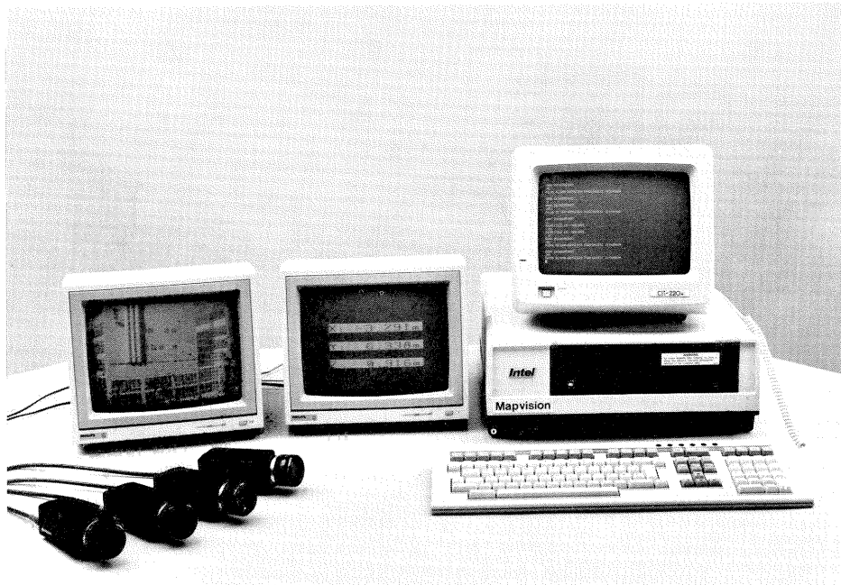
Figure 3. The Mapvision is a stand-alone photogrammetric machine vision system especially developed for industrial inspection and assembly control applications.
