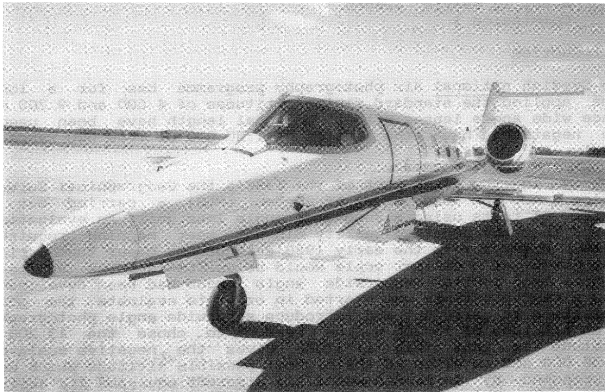
Figure 1. Aircraft of the Lear Jet 35 type used for aerial photography at 13 200 m. The plane is equipped with a special door housing the camera.
