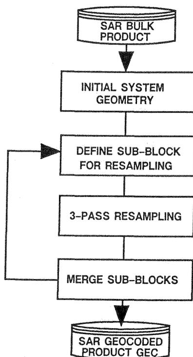
Figure 1. Geocoding Process without DEM Correction
