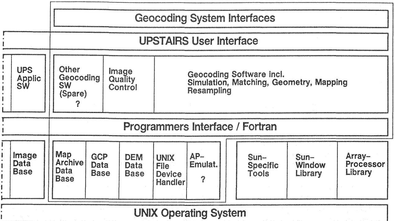
Figure 3. Geocoding Image Processing System Software Layers
