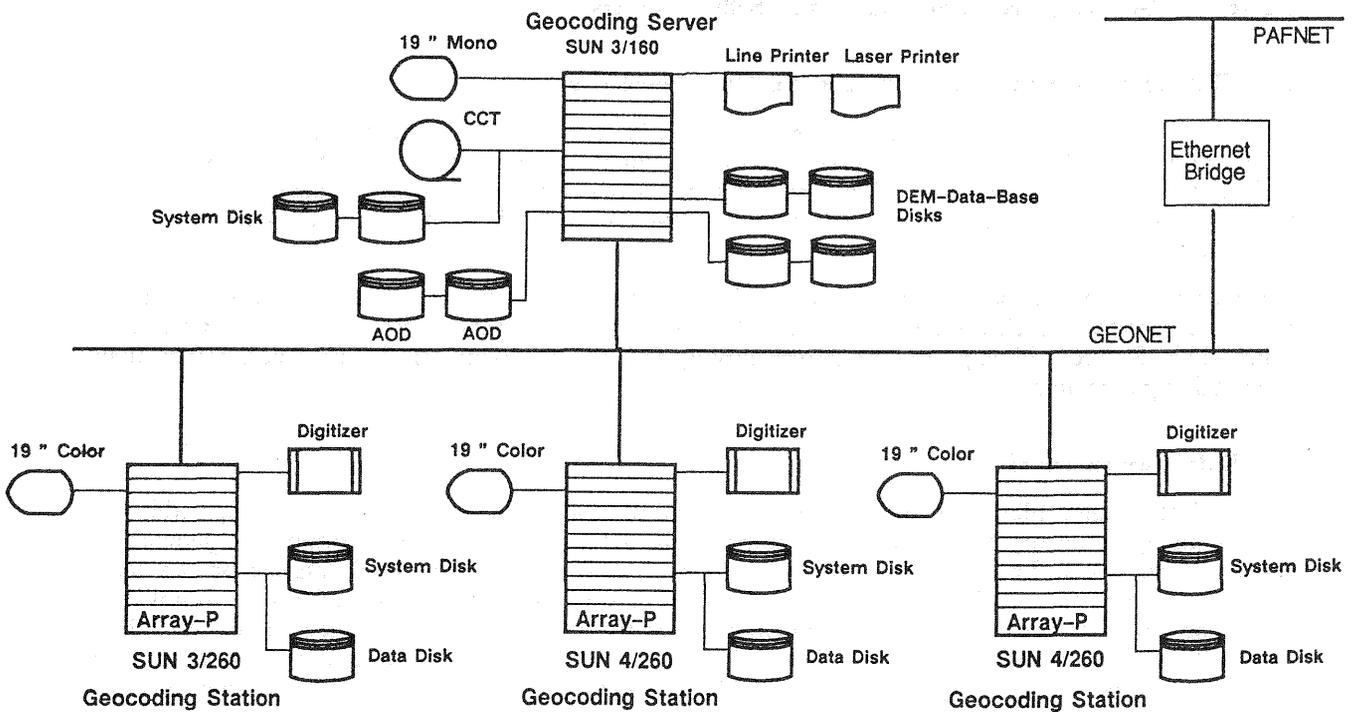
Figure 4. Hardware Configuration of the Geocoding System
