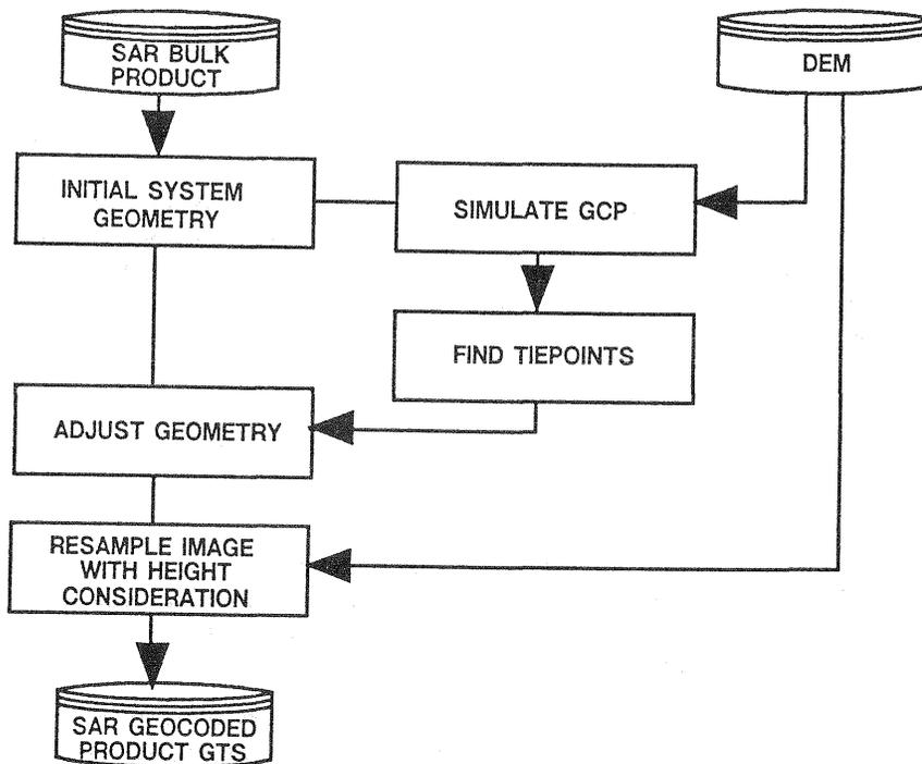
Figure 2. Geocoding Process with DEM Correction
