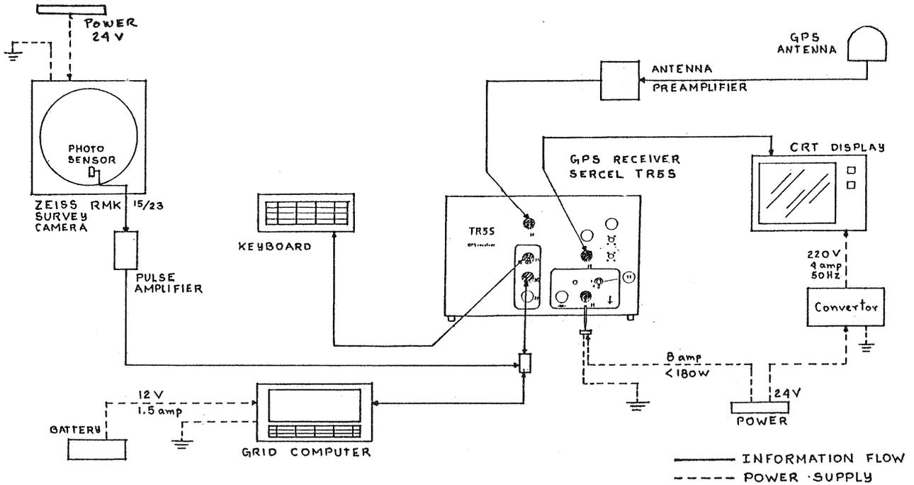
Figure 1. Integrated system configuration.
