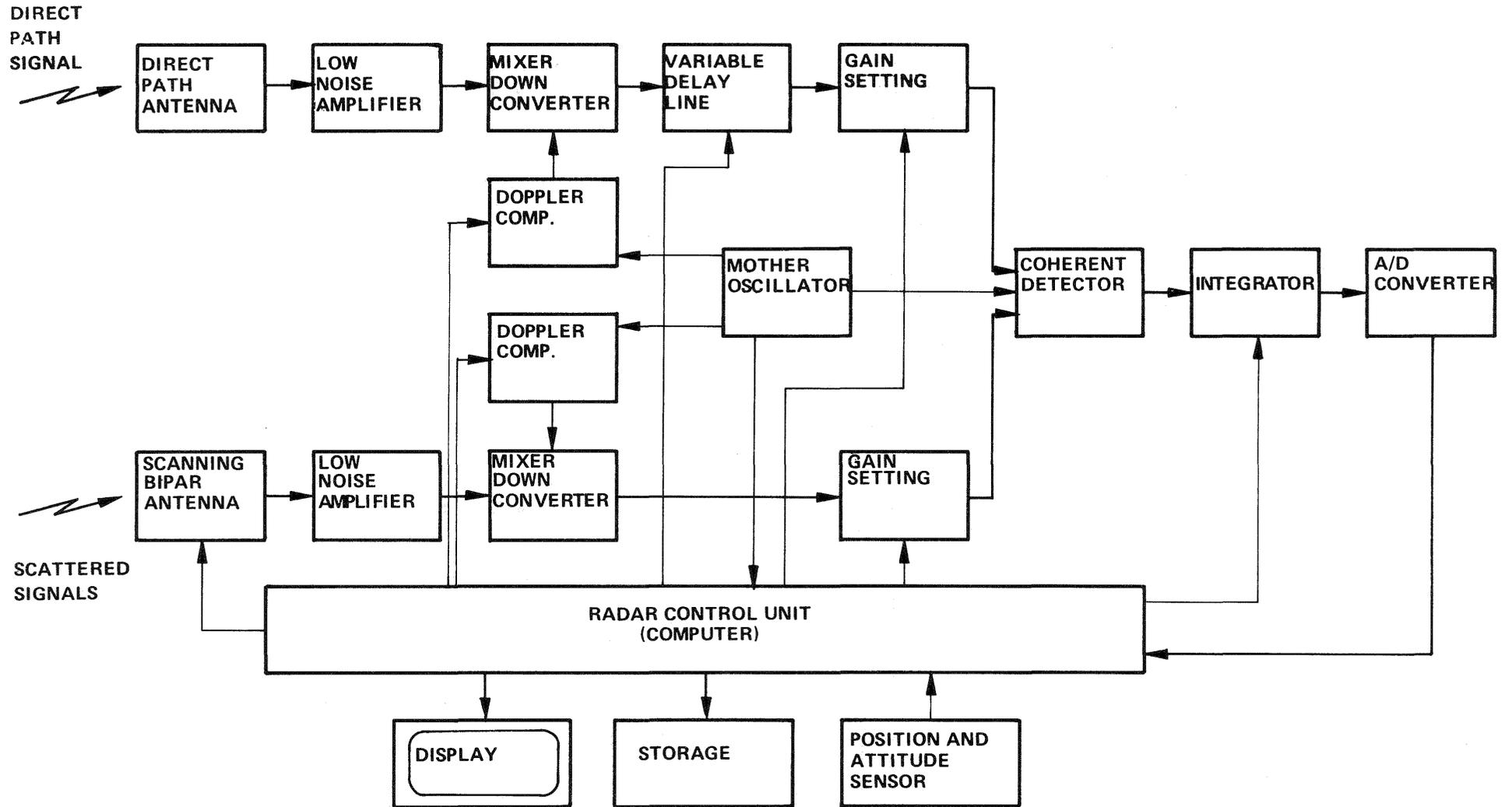
Fig. 2: Block diagram of a BIPAR receiver
