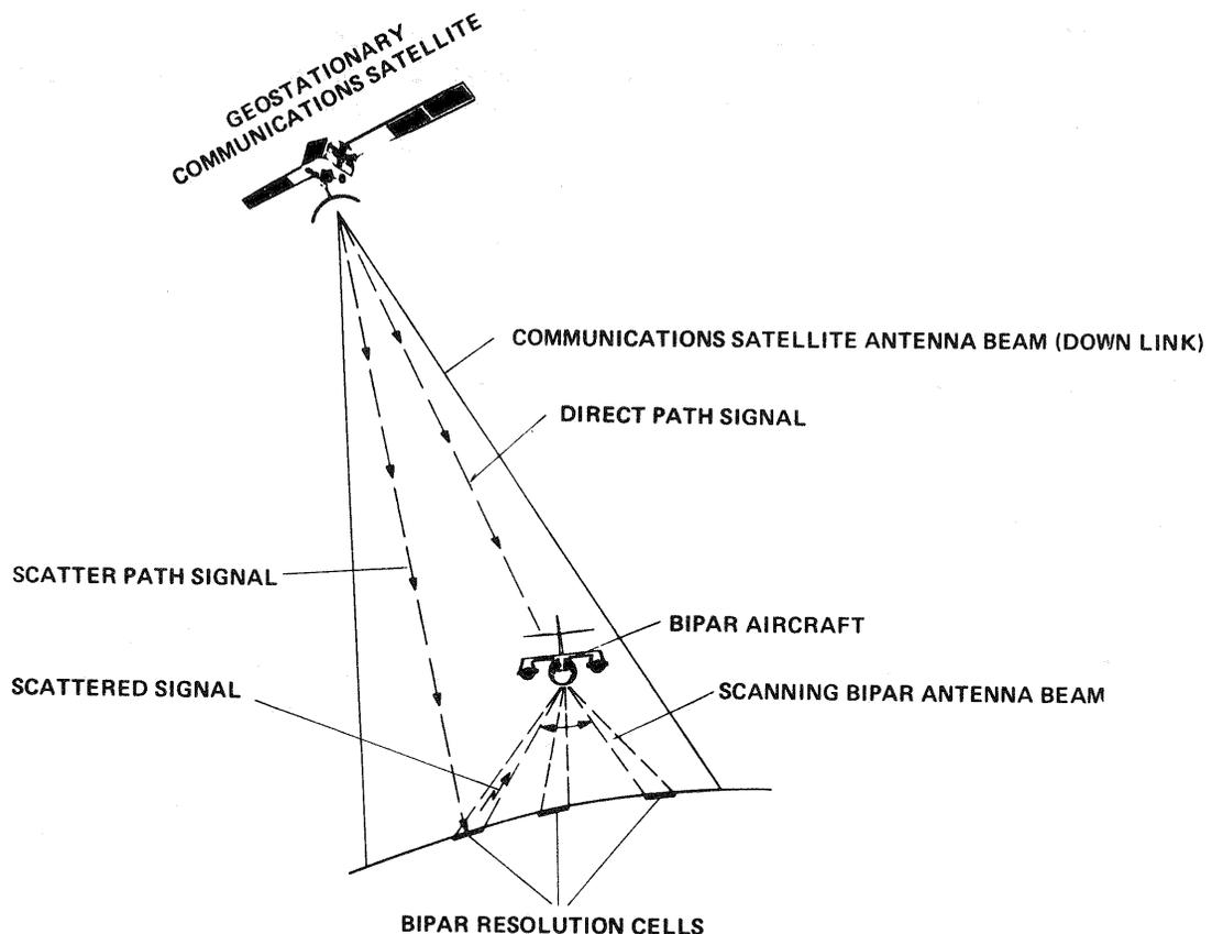
Fig. 1: Typical BIPAR System Geometry
