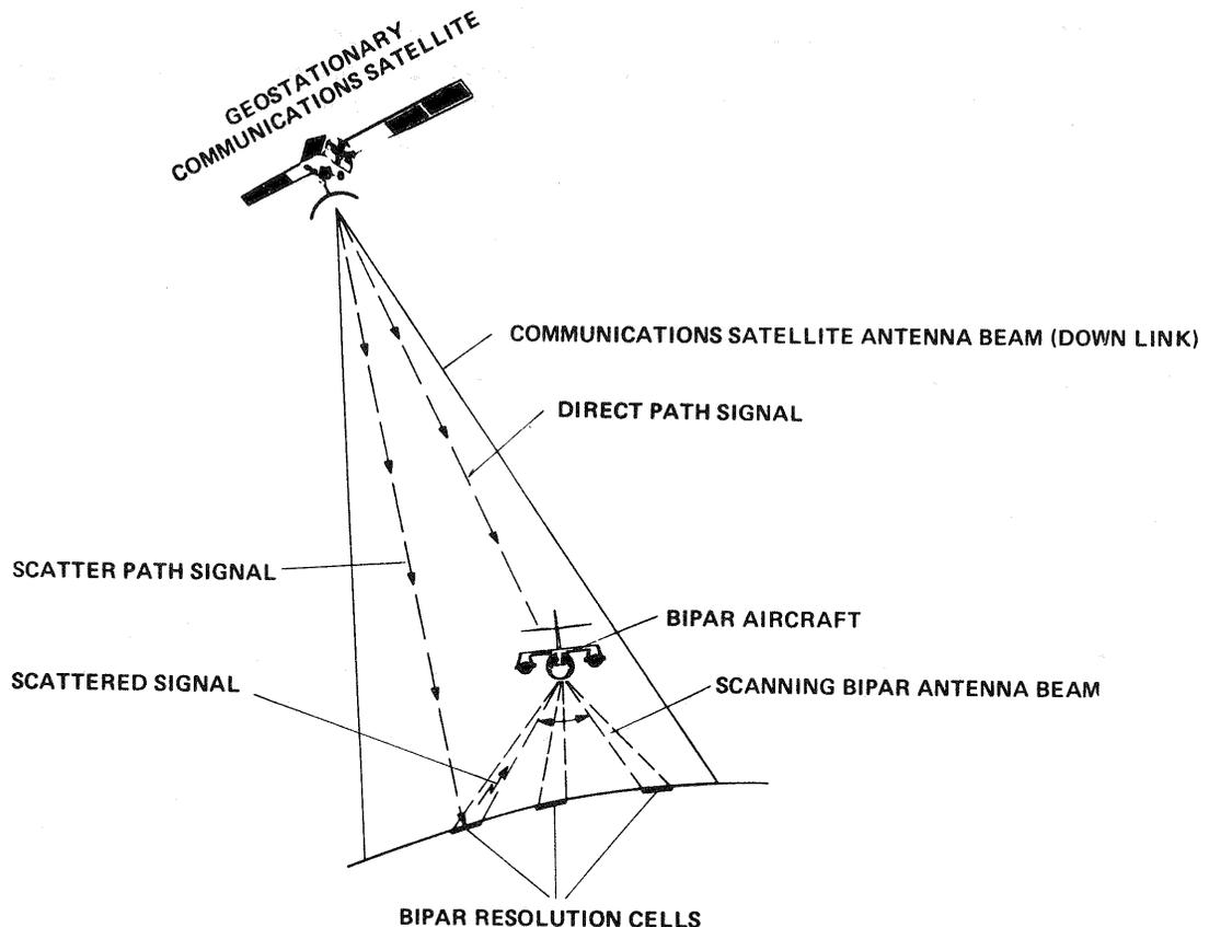
Fig. 1: Typical BIPAR System Geometry
