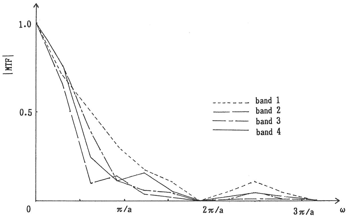
Fig. 5 Estimated MTF of the MESSR on the MOS-1 satellite
