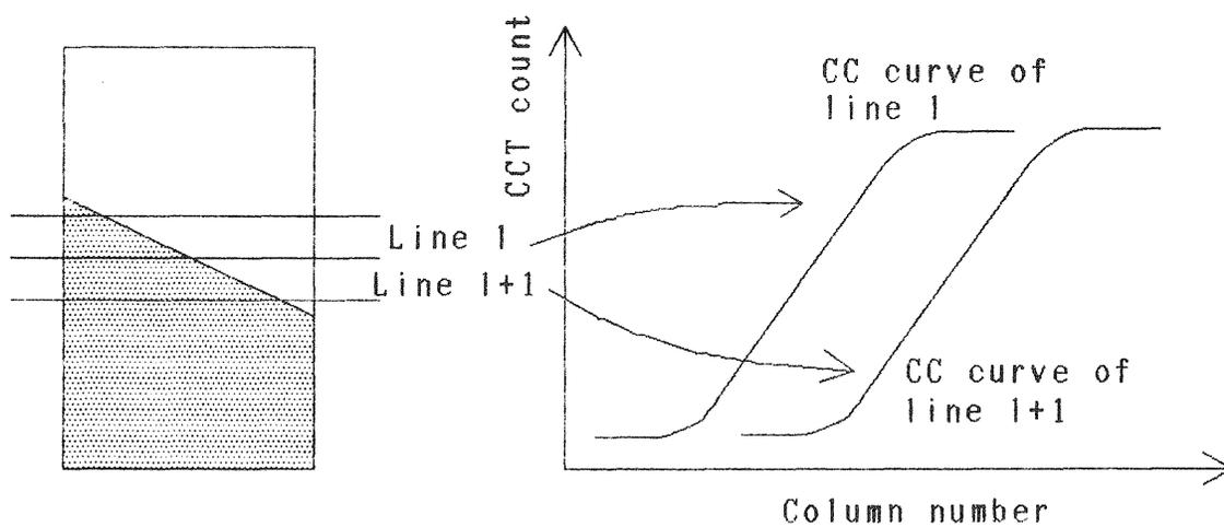
Fig. 3 CC curve of line l and l+1
