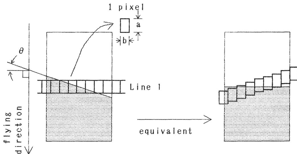
Fig. 1 Basic idea of the PSF measurement
