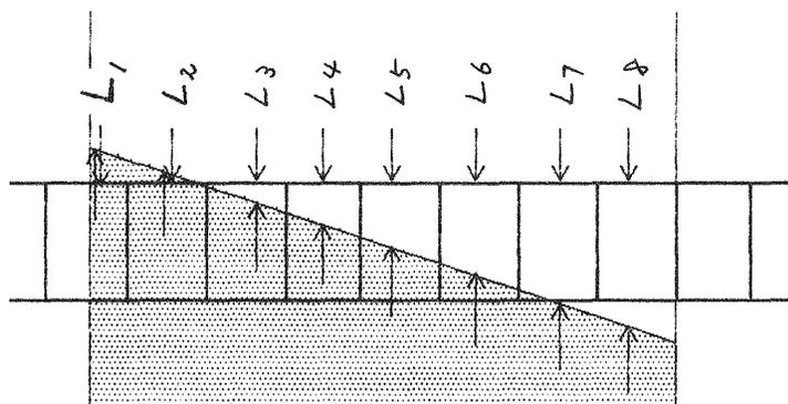
Fig. 2 Relative locations of pixels to the edge
