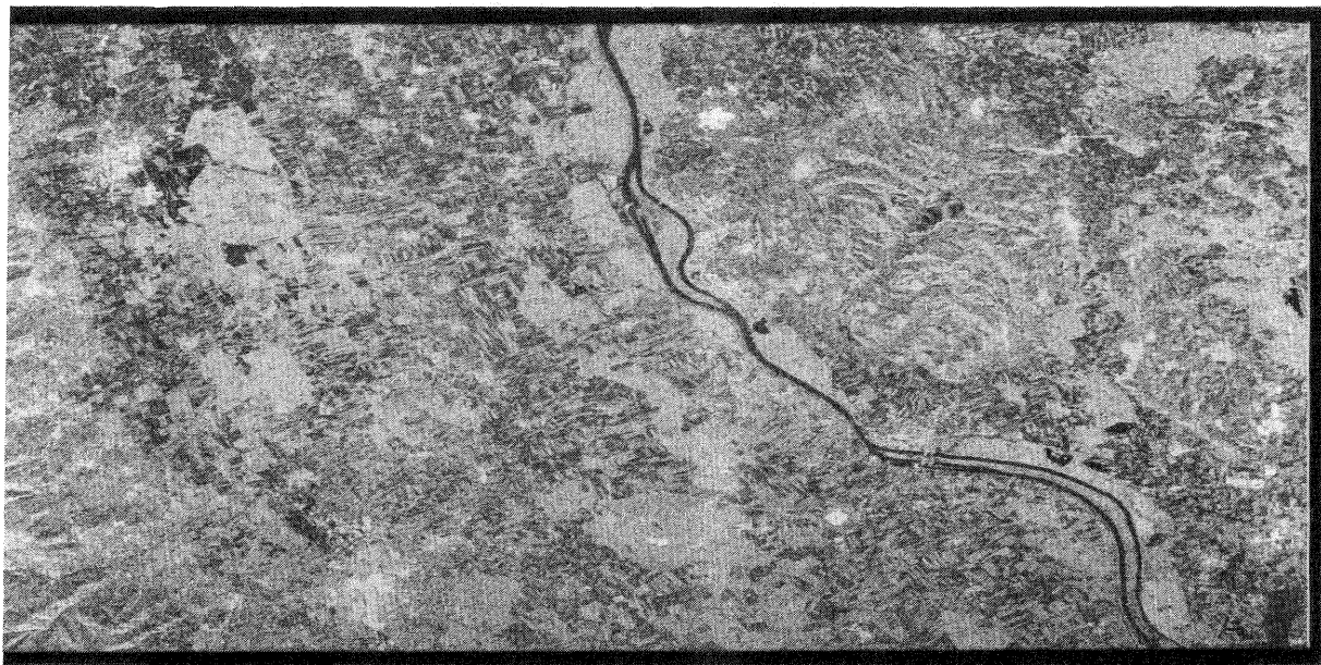
Fig. 4.4: Spaceborne SAR ground range image of the Freiburg test site (approximate scale 1 : 200 000)
